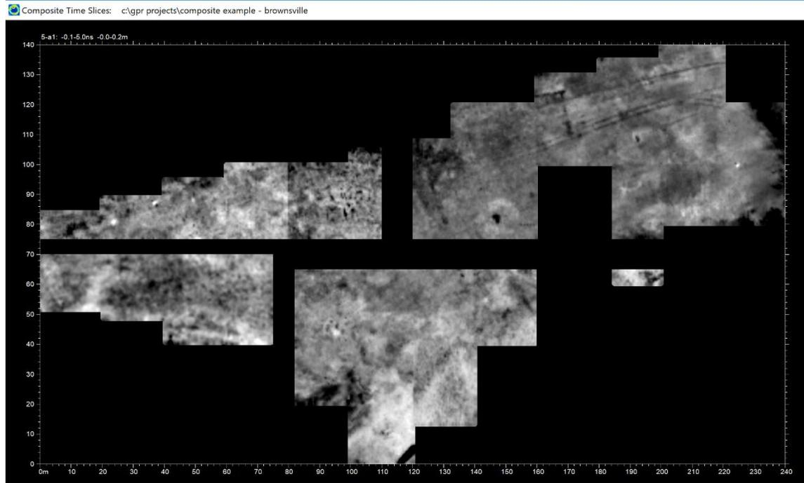
Figure 3. Example of the Composite time slice menu at a site in Brownsville, TX. (data courtesy of Steve DeVore, National Park Service)
