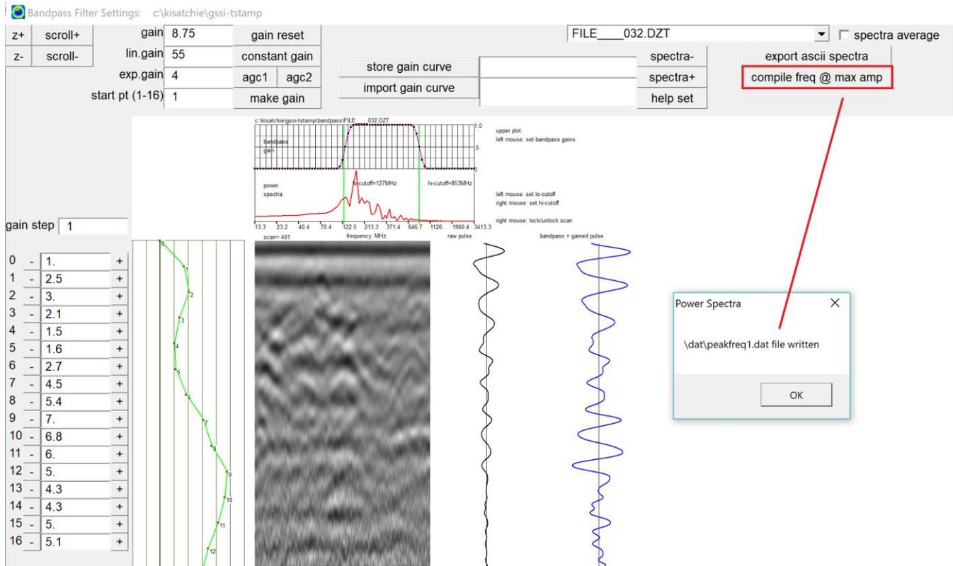
Figure 1. Location of the new operation to compile the frequency at maximum amplitude in the Spectra+Gain menu.
