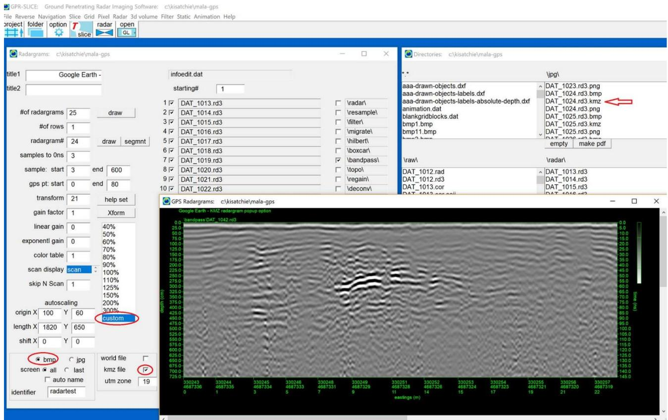
Figure 5. Settings in the Radar 2D menu needed to create KMZ popup radargrams. KMZ popup files can be generated in batch.
