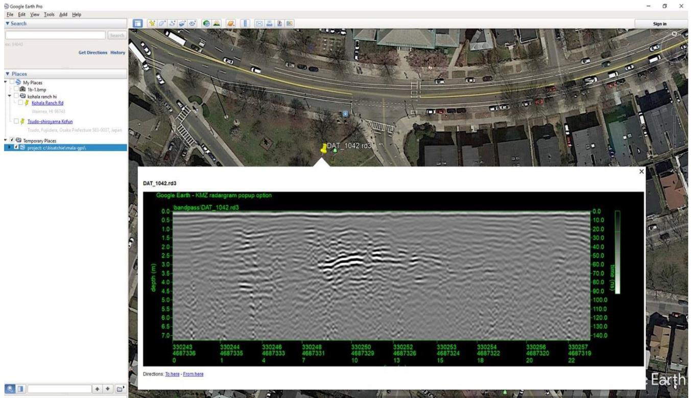
Figure 6. Example of a KMZ popup 2D radargram in Google Earth. The user must click on the yellow pin to see the associated image appear.
